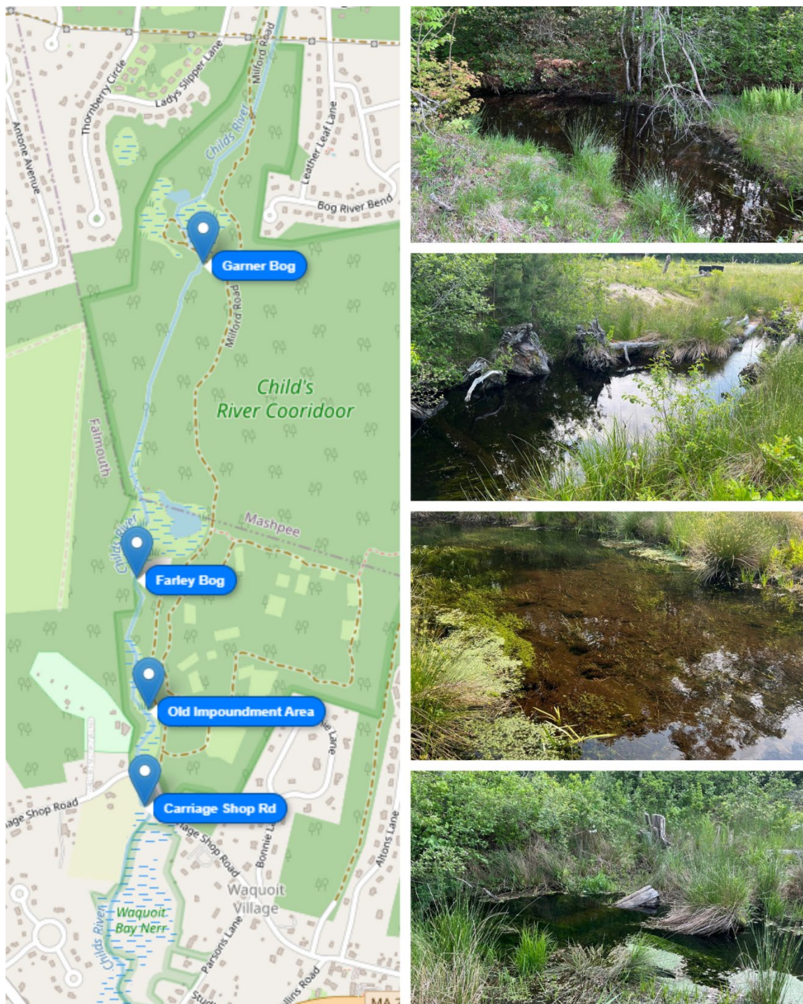
Figure 3. Map (left) showing the locations of the four sediment traps installed as part of the Childs River restoration design. These structures help manage sediment loads and reduce siltation in sensitive habitats, supporting the long-term success of the restoration effort. Photos of each sediment trap are shown on the right, ordered from north to south along the restored channel.
